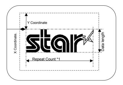
\*1: The following equation is for the number of times to repeat the command (when the image data count is an integer magnification of the data length).
